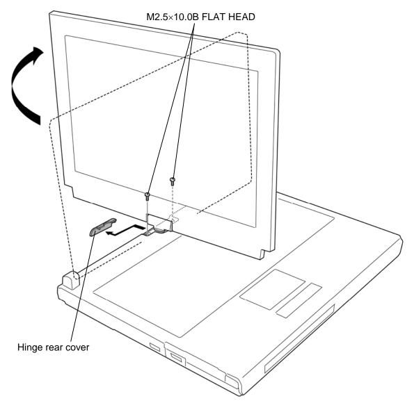
Figure 4-25 Removing the base assembly and cover assembly (2)
